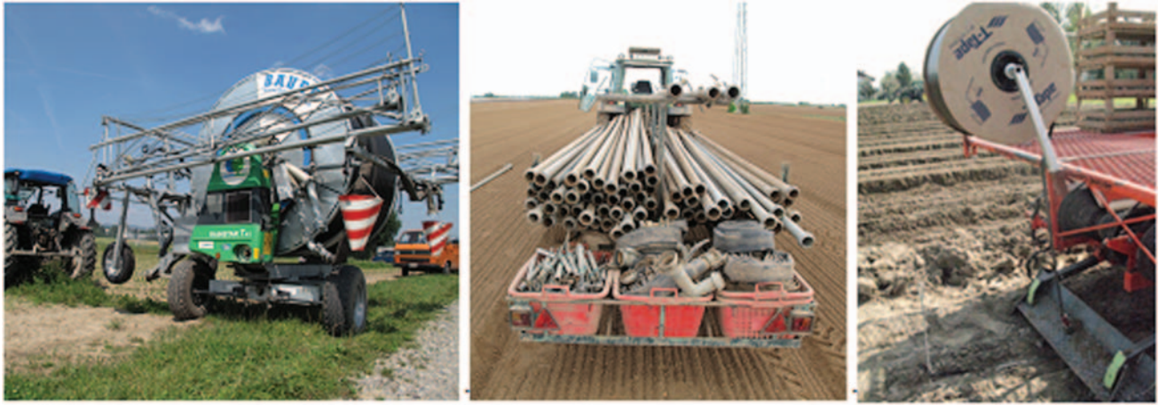
Figure 2: Mobile sprinkler (Rollomat) (left), Assembly of fixed sprinkler (centre), Laying of drip irrigation (right) (source: Agroscope)
