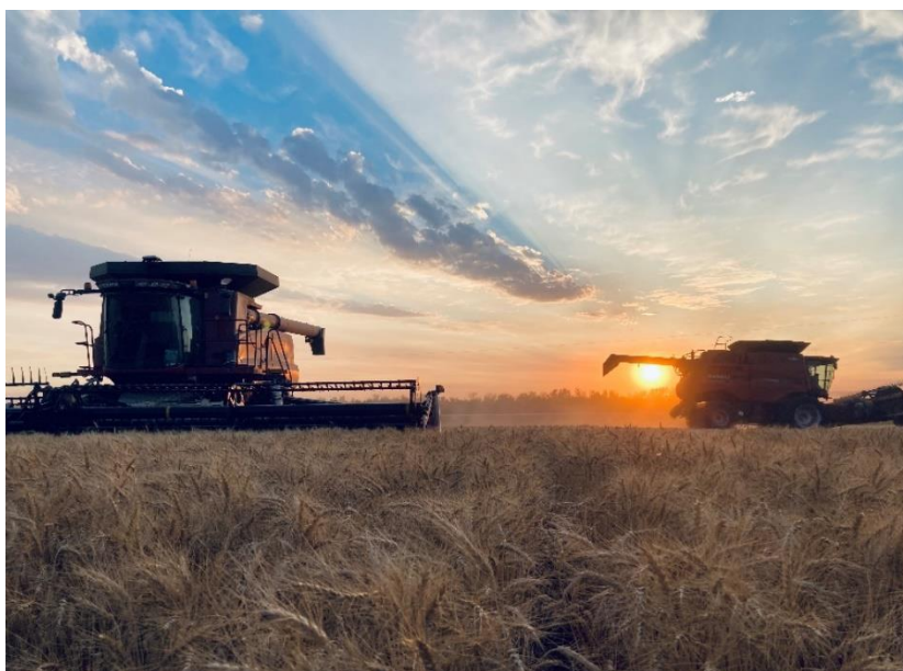
Two Case IH axial flow combines (9230 and 9240 models) with 40ft flex draper headers harvesting hard red spring wheat at sunset.
